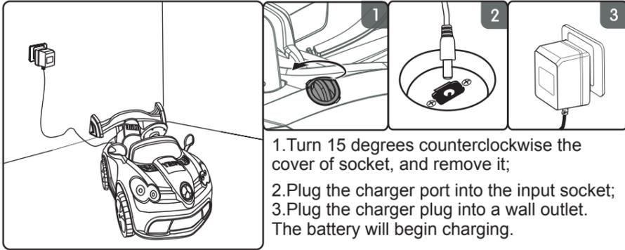
1. Turn 15 degrees counterclockwise the cover of socket, and remove it;
